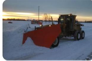
While a motor grader is not as efficient as a regular snowplow truck, the advantages of more horsepower and traction make it a valuable piece of equipment for various
