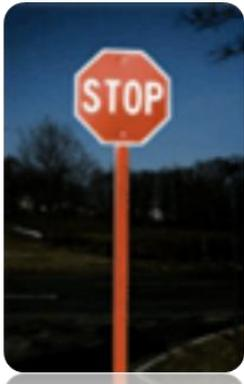
Shown above is a reflective panel installed on a stop sign post.
